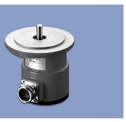
Using this potentiometer a maximum angular rotation of 3800° can be converted into a voltage proportional to the angle of rotation, through the medium of a conductive-plastic potentiometer.
